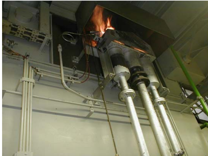
Picture 8: burning system at a multipurpose chamber furnace type MKG
