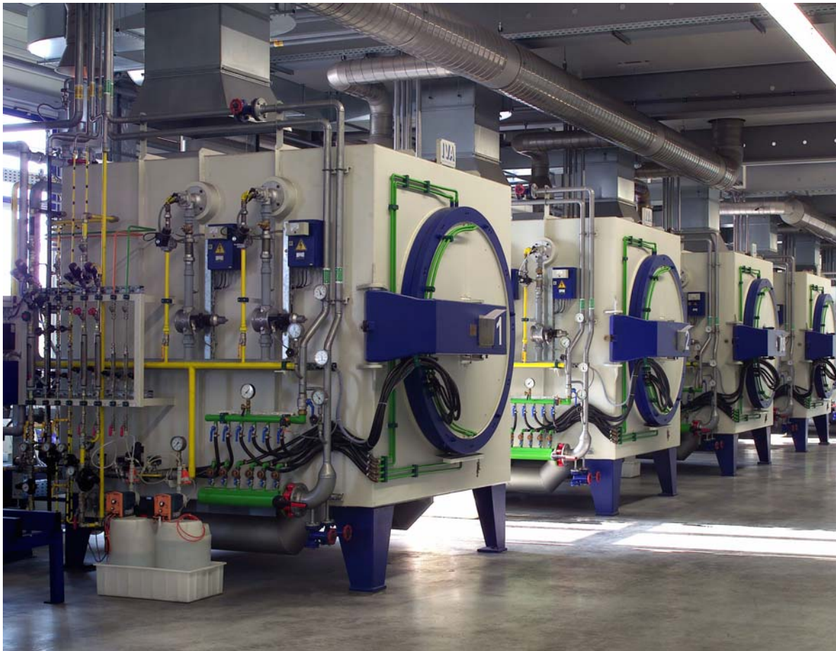
Picture 1: gas heated, evacuable nitriding furnaces type RH... RV/g, the plastic containers for water and CITROX®- solution can be seen in the left lower corner of the picture
