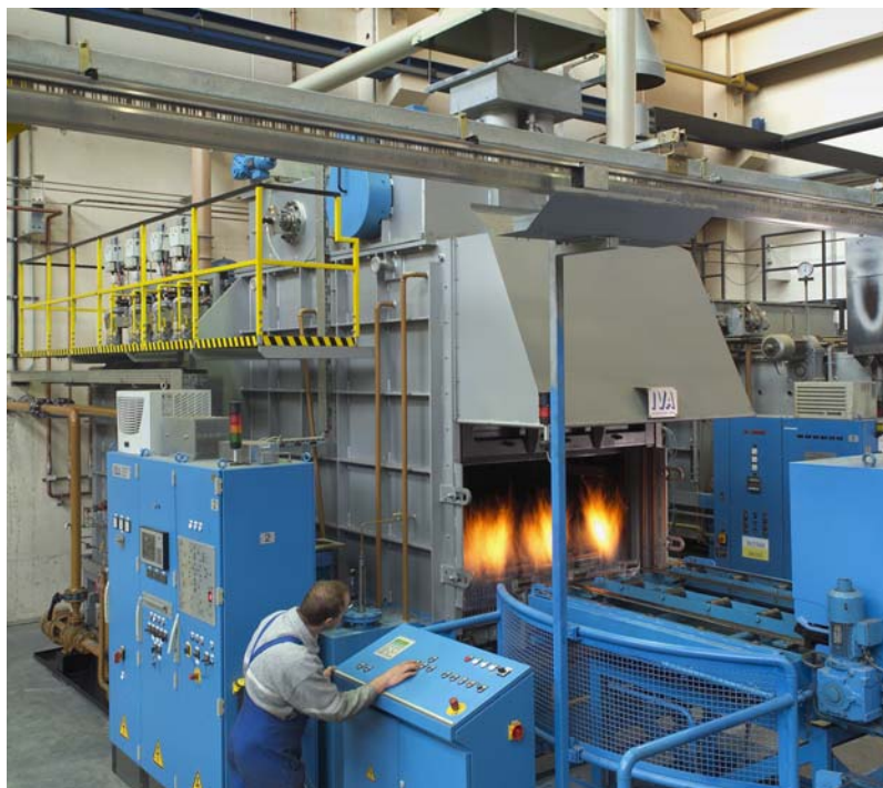
Picture 9: multipurpose chamber furnace type MKG
